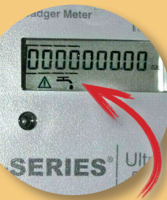
On new digital meters the leak indicator is a faucet icon.
